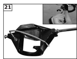
Install two screws corresponding with the "L" shaped holes in the canopy only part way so that canopy can twist into place. Remove the all thread studs from the lower part of the mounting bracket.
